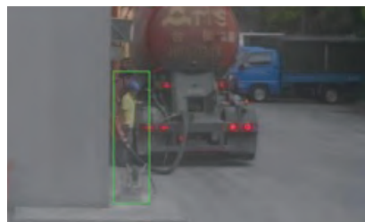
↑ AI Image Recognition Detected personnel not wearing a safety helmet and reflective vest, immediately issued a warning.
