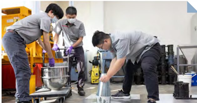
Test for slump flow of UHPC
