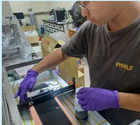
Electrode sheet production process: Battery slurry is placed on copper sheets and pressed into electrodes using a rolling press.
